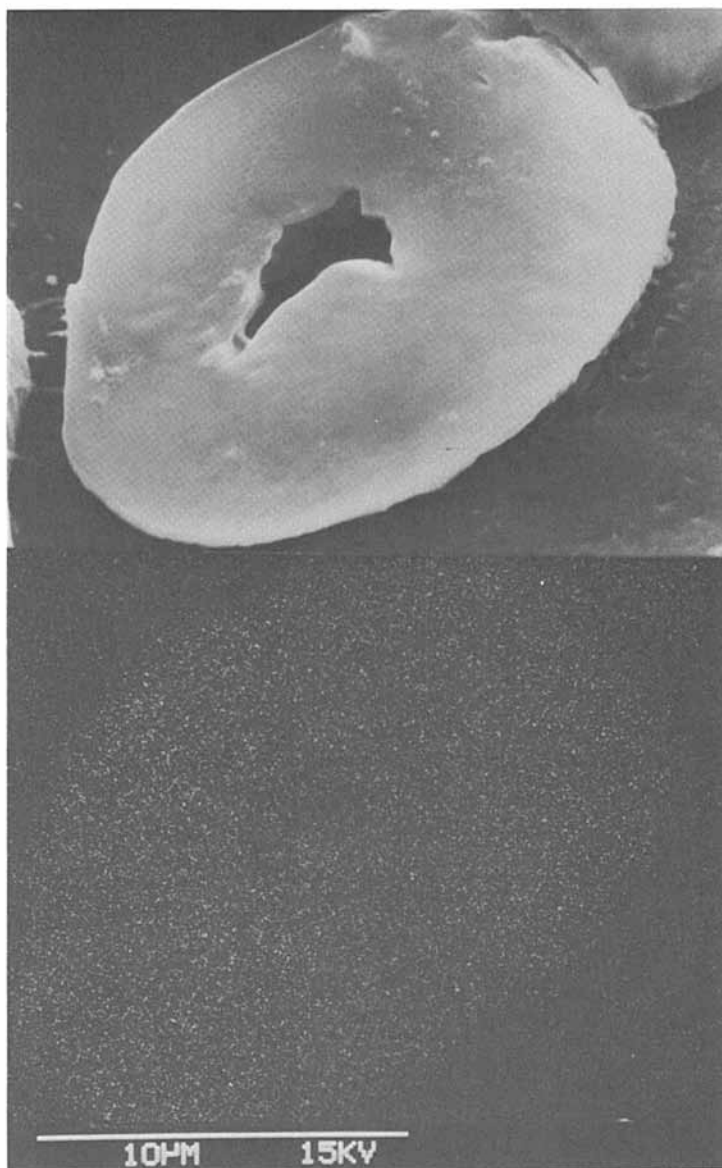
Figure 10. Scanning electron micrograph of a cross-section (top) of a diquatery ammonium cellulose prepared by reaction of a DEAE cellulose (2.57% N) with diiodopentane and exchanged to thiocyanate form (100% conversion) and EDAX (bottom) showing distribution of S throughout fiber.
