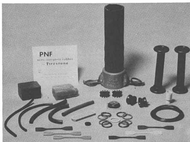
Figure 5. Phosphazene fluoroelastomer (PNF) compounds were used to prepare molded rubber parts for diverse applications. Shown here include O-rings fuel hoses, shock absorption and vibration damping mounts. Photograph courtesy of the Firestone Tire and Rubber Co.
