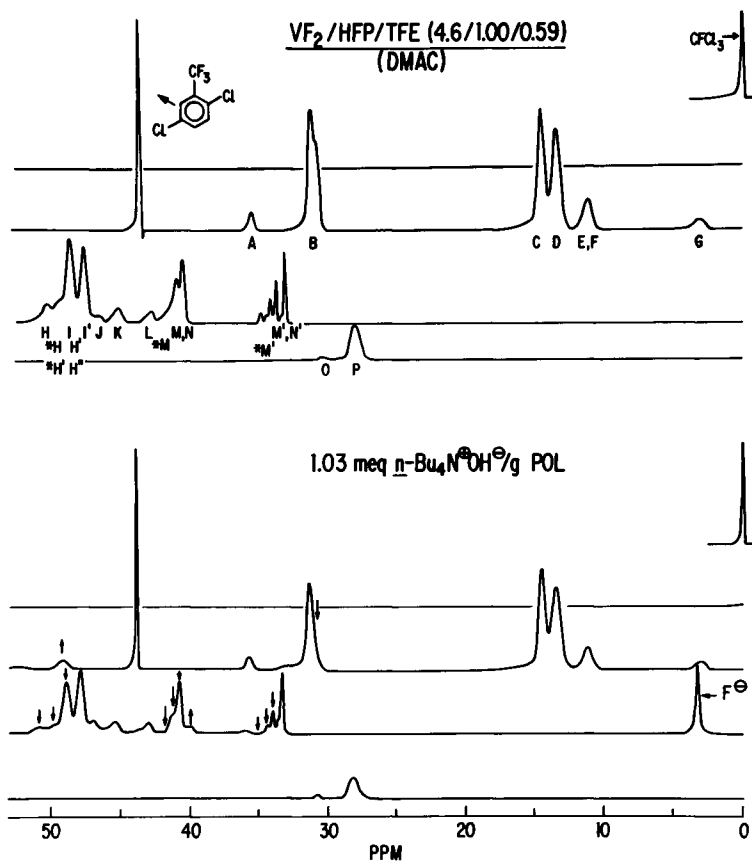
Figure 8. 94.1 MHz ^{19}\text{F} NMR spectrum of a VF 2 /HFP/TFE polymer in DMAC before (top) and after (bottom) treatment with a hydroxylic base.
